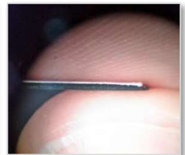
Printer Paper (White) and TiVC (black) between fingers under magnification
