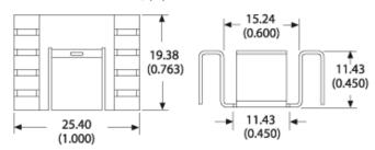
Recommended copper pad size for heat sink and device mounting footprint
